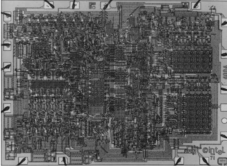
■ FIGURE 1-3 The 4004 Intel microprocessor [9].
