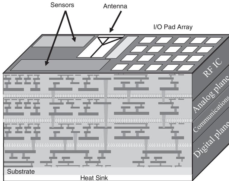
■ **FIGURE 1-9** An example of a heterogeneous 3-D system-on-chip comprising sensor and processing planes.
