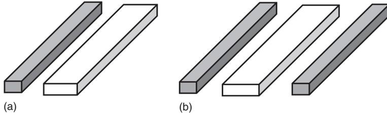
■ FIGURE 1-6 Interconnect shielding to improve signal integrity: (a) single-sided and (b) double-sided shielding. The shield and signal lines are illustrated by the grey and white color, respectively.
