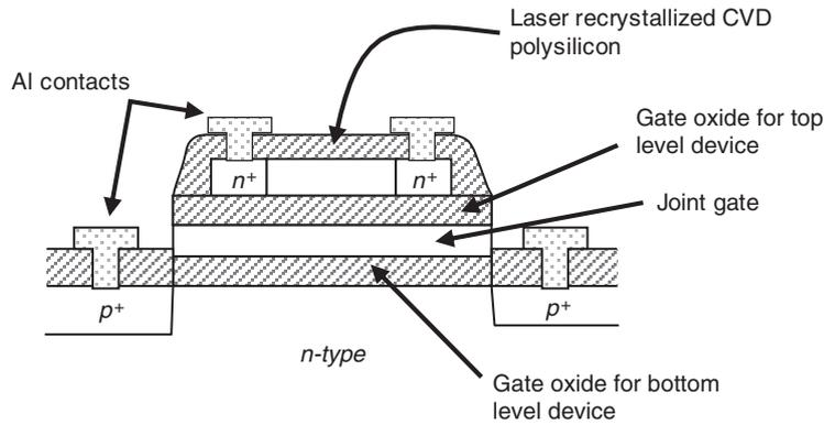
■ FIGURE 1-7 Cross section of a JMOS inverter [35].
