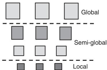
■ FIGURE 1-4 Interconnect architecture including local, semi-global, and global tiers. The metal layers on each tier are of different thicknesses.
