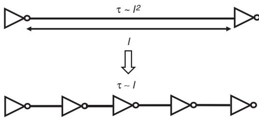
■ FIGURE 1-5 Repeaters are inserted at specific distances to improve the interconnect delay.
