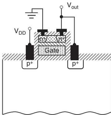
■ FIGURE 2-1 Three-dimensional stacked inverter [34].
